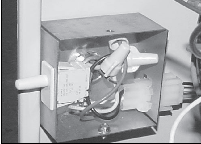
FIGURE 34 - INTEGRATED HOT SURFACE IGNITION CONTROL
